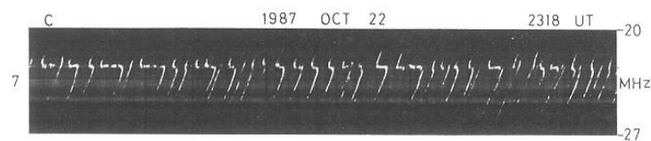
Figure 4: The narrow-band disappeared and only the Riihimaa structures are observed
