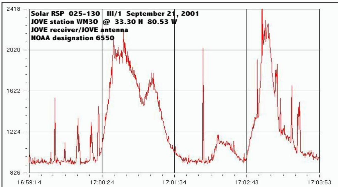
Type IV events are a smooth continuum of broadband bursts primarily in the meter range (300-30 MHz). These bursts occur with some major flare events; they begin 10 to 20 minutes after the flare maximum and can last for hours.
